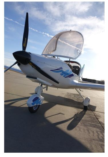
Empty weight 780 lbs Max Weight 1320 lbs Fuel Burn 4 gph Endurance 7.5 hrs Cruise Speed 115 kts Landing Roll 345 ft Stall Speed 39 kts Vne 164 kts
