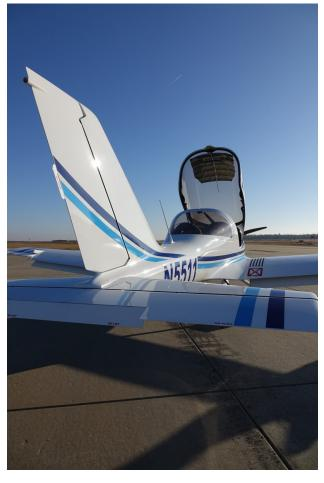
Empty weight 780 lbs Max Weight 1320 lbs Fuel Burn 4 gph Endurance 7.5 hrs Cruise Speed 115 kts Landing Roll 345 ft Stall Speed 39 kts Vne 164 kts
